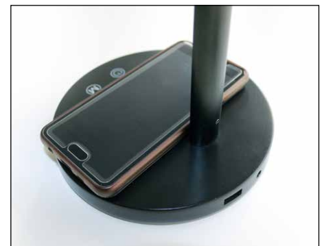
Inductive charging pad in the base
